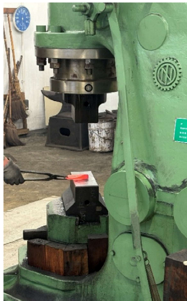
Fig. 2.2.1 Picture of forging by air hammer
